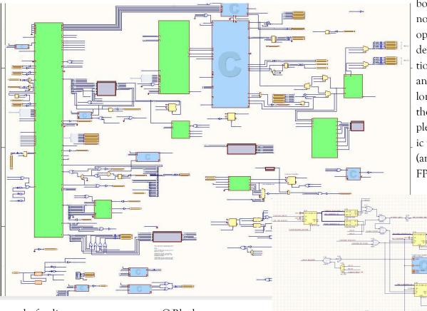
board. Although I cannot divulge too many operational details, I will describe some of the sections of the schematic and their purpose. The long green rectangle on the left is actually a completely separate schematic which contains (among other things) an FPGA "soft processor".
