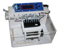
This product was designed and sold by C-Horse Software, Inc. It is designed to clean inkjet heads. It was specifically designed to clean the Epson DX5 head which was and still is, a very popular head for re-purposed direct-to-garment applications. It has been known to revive print heads that would have otherwise been deemed "unrecoverable"
