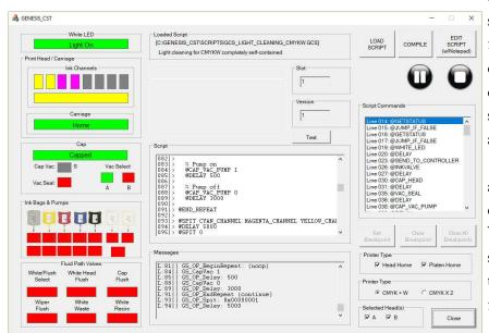
etc. per test iteration can be very time consuming when defining the routines. For this reason, I designed a scripting system. The core firmware has default cleaning routine code which it defaults to, however, cleaning scripts can be downloaded to overwrite or add cleaning routines.
