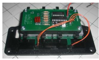
This hardware module was designed for specialty printers based on the Epson Stylus Color R1900. These printers normally used bulk-ink supply tanks instead of cartridges. For this reason, modules are used which simulate a full cartridge. These modules are typically reset by hand with a built-in button whenever they read empty. The C-Set module was designed to make it possible for
